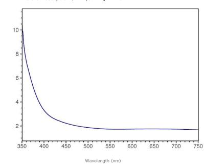
**Transmission absorption spectra** in the UV to near-IR range (250-1000 nm) were collected using a Hitachi U4001 spectrometer (2.0 nm slit, 1.0 nm data interval, and 120 nm/min scan speed). Unless otherwise noted, an unpolarized light beam was focused on the culet area of the optically unoriented sample.
