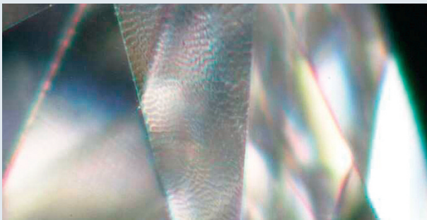
Lizard skin: transparent uneven texture confined to one facet; caused by polishing a facet off-grain, at the hardest direction near a cleavage plane.
